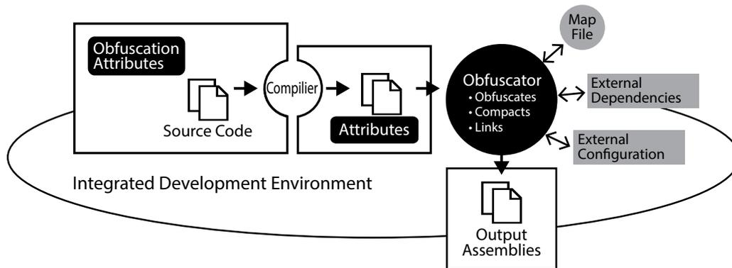
**Figure II: Application Hardening Development Process**
